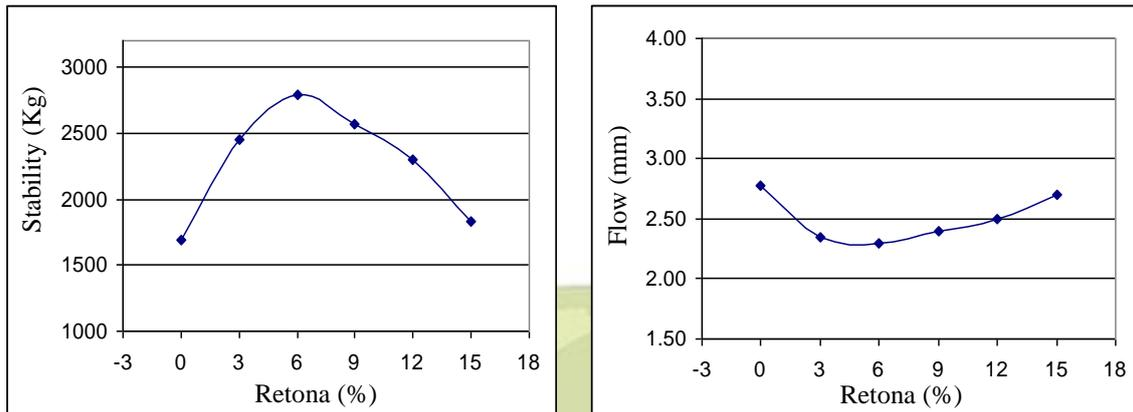
Figure 1 Stability and flow of mixture at different Retona content
