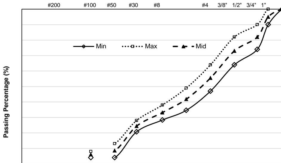
Figure 1. Aggregate Grading Specification and Design
