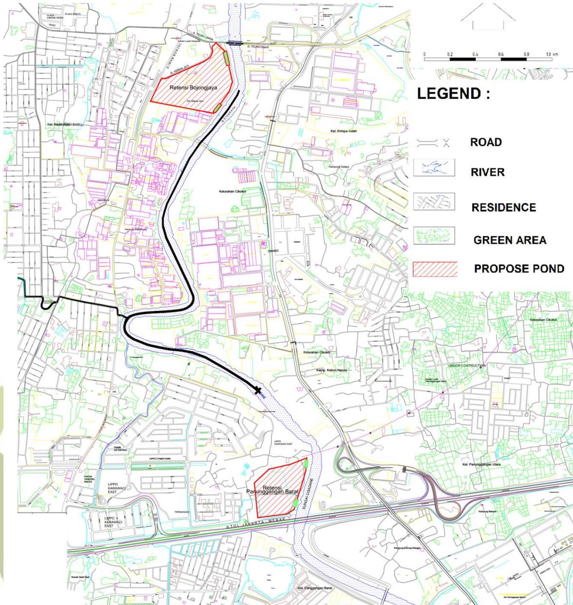
Figure 9 Alternative Location of Tapping Raw Water at Cisadane Tangerang City
