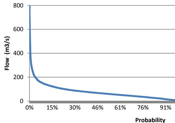
Figure 2 Flow Duration Curve of Cisadane at 90% Confidence Level
