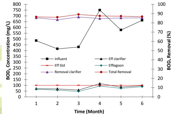
Figure 4 Concentration and removal of BOD<sub>5</sub>
