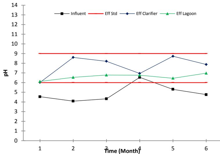
Figure 1 pH of the influent and effluent
