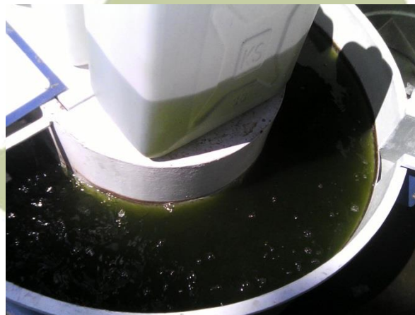
Figure 2 Running Oxidation Ditch Algae Reactor (ODAR)
