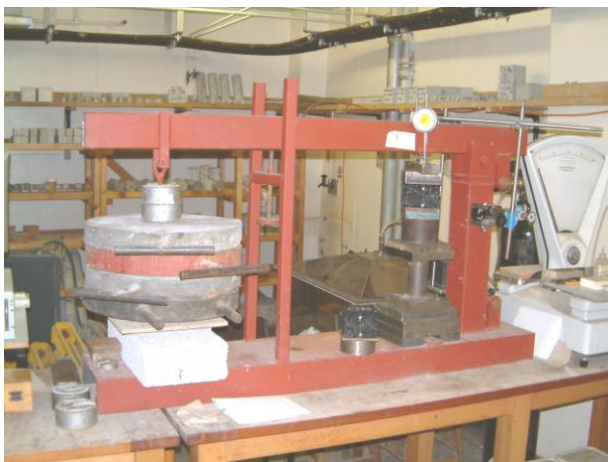
Figure 6. Arm load machine used for creep test loading
