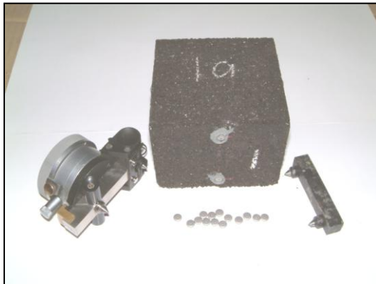
Figure 5. The CDWblock sample and strain measuring equipment
