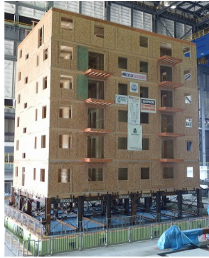
Figure 6. Steel ground + 6 story light timber framing test specimen on the shaking table of E-defense.
