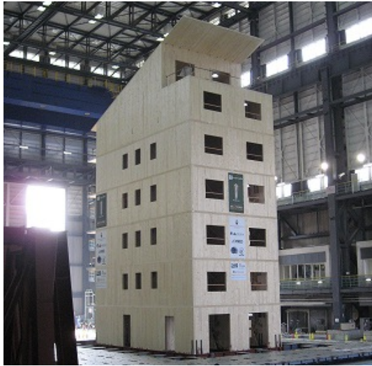
Figure 5. Story CLT test specimen on the shaking table of E-defense.
