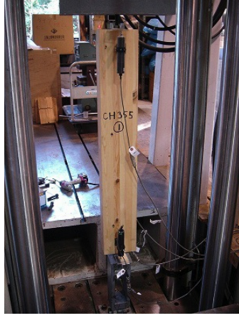
Figure 21. Pull-out strength experiment of single LSB joint penetrated parallel to the grain of glulam.
