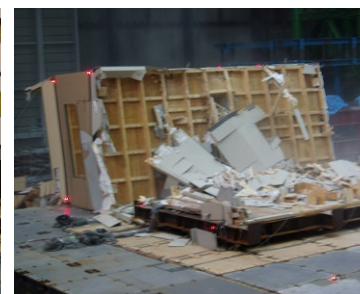
c) Close-up view of collapsed specimen. It was shown through this sensational experiment that the prediction of collapse on full scale wooden dwelling house was not so straightforward.
