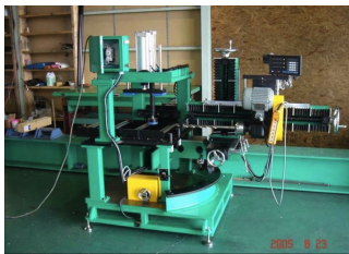
Figure16. Specially designed bowling machine and high power torque wrench for LSB. (Courtesy of Gradworks Co. Ltd.)
