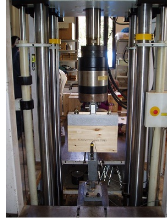
Figure 22. Pull-out strength experiment of single LSB penetrated perpendicular to the grain of glulam.
