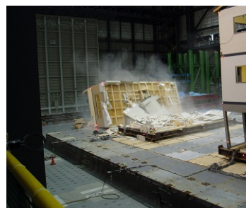
b) Specimen anticipated to be survival was first collapsed out of prediction. While that anticipated to be collapsed remained without fatal collapse.
