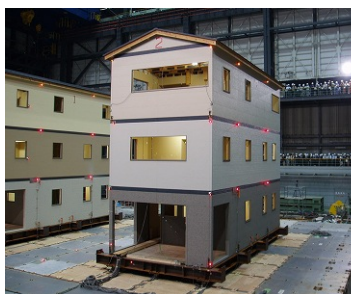
a) Three story wooden post & beam house on shaking table facility. Two specimens were put on the table and Kobe earthquake record was given to them at the same time.
