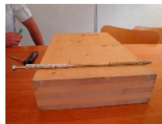
b) Cross Laminated Timber (CLT) and long screw used for constructing 9-storey building at London.
