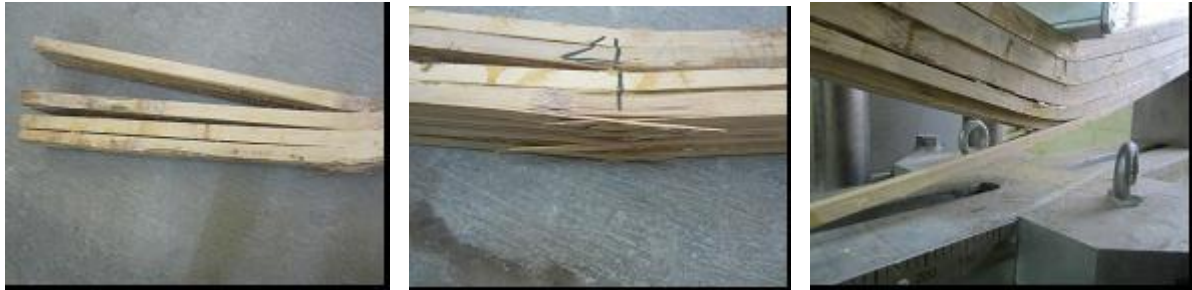
(a). slip at glued surface (b). simple tension at bottom lamina (c). horizontal shear
