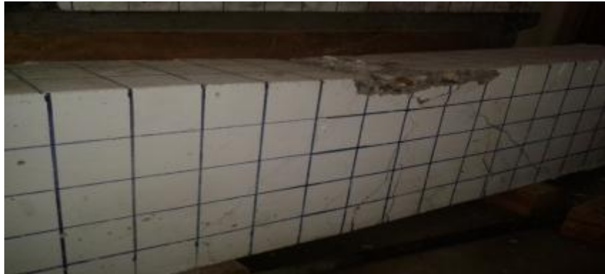
Figure 6. Flexure failure at specimen
