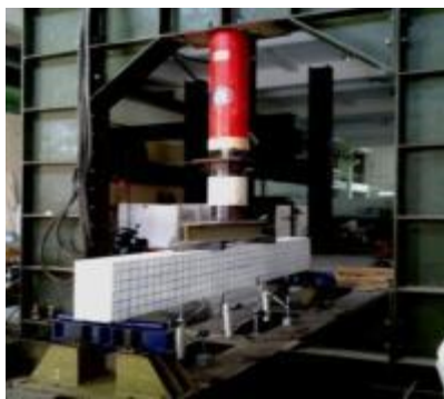
(a) Beam installed in loading frame
