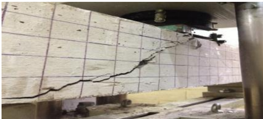
Figure 7. Shear failure at specimen
