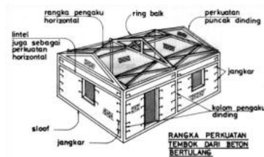
Figure 4. Connectivity among building components (Source: Dirjen Cipta Karya, 1993)
