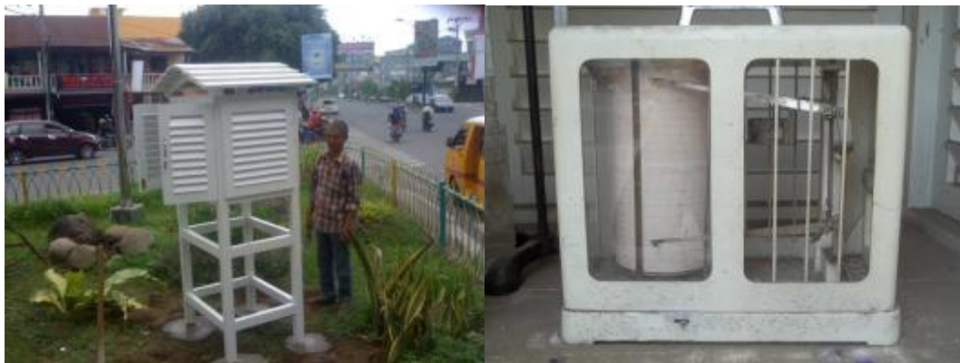
Figure 1. Stevenson screen situated in the node of shop house district (left) and the thermo-hygrograph inside it (right)
