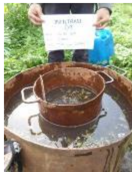
Figure 4. Double Rings Infiltrometer for Insitu Infiltration Measuring
