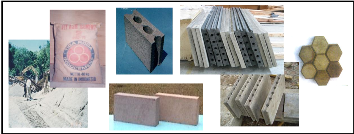
Figure 2. building components from RCC (waste of oil)
