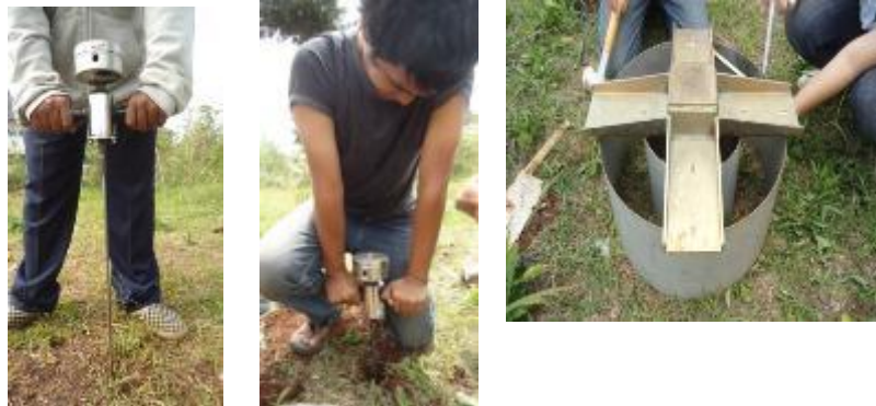
Figure 6. The Measurements of Soil Hardness and Infiltration around the LRB.
