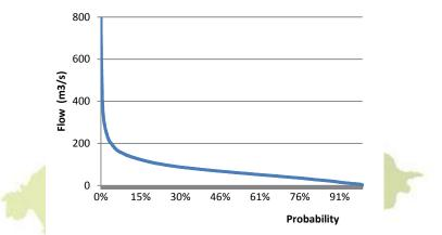
Figure 2 Flow Duration Curve of Cisadane at 90% Confidence Level
