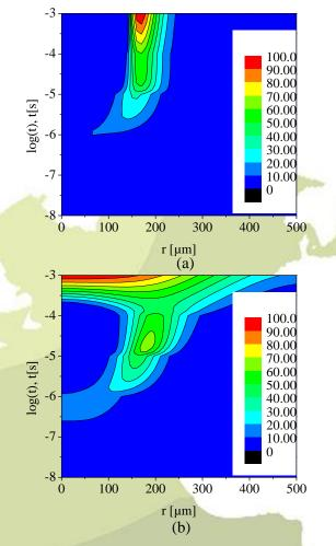
Figure 4: NO<sub>2</sub> radial profil evolution (a) without diffusion ( $n_{max}$ =32.4 ppm ;  $n_{min}$ <0.001 ppm); (b) with temperature variation and diffusion effects ( $n_{max}$ =20.7 ppm ;  $n_{min}$ <0.001 ppm)
