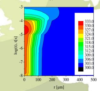
Figure 2: Radial gas temperature profile evolution (units in <sup>o</sup>K)
