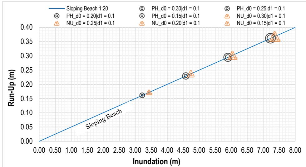
Figure 5 Relation between run-up and maximum inundation based on physical and numerical model. Higher  $d_0$  is indicated by larger symbol
