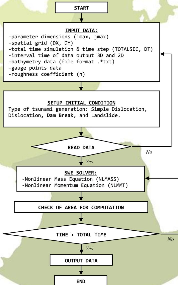
Figure 3 Flowchart of tsunami simulation using TUNAMI Modified (beta version)
