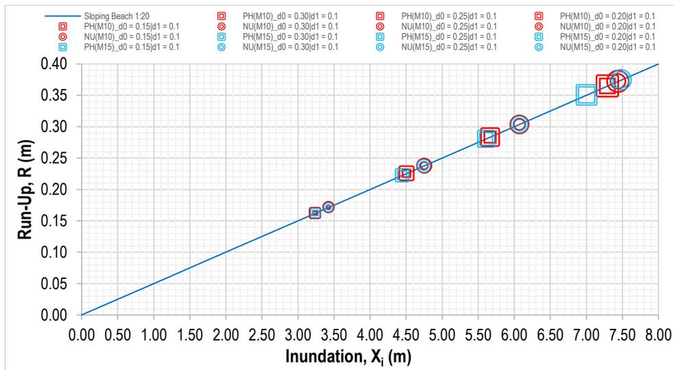
Figure 8 Effect of two types of square building over the run-up and inundation variable
