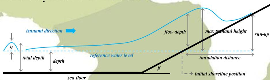
Figure 2 Sketch of tsunami terminology for the wave climbing up a sloping beach
