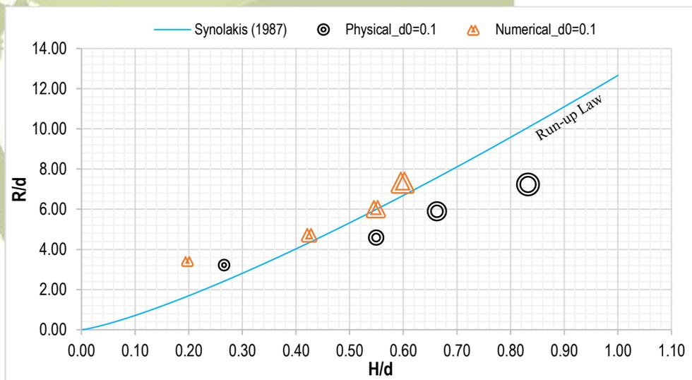
Figure 6 Relation between non-dimensional parameter  $R/d$  and  $H/d$  together with the run-up law (Eq. 1). Higher  $d_0$  is indicated by larger symbol
