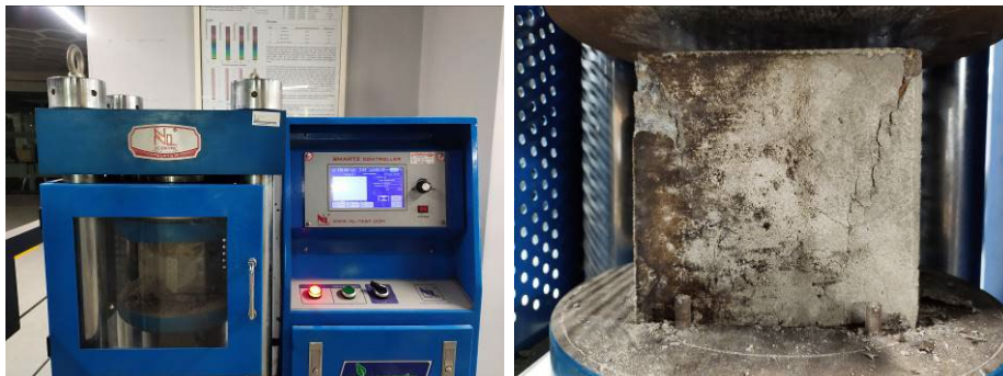
Figure 4. An experimental test for compressive strength of concrete
