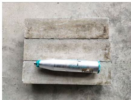
Figure 5. Rebound strength inspection of nano concrete
