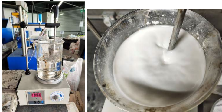
Figure 1. Magnetic stirrer with nano-dispersion
