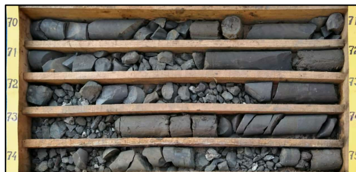
Figure 2. Sample of core drill data at BTS-2 (poor rock quality) (PT Wahana Adya Konsultan, 2019)
