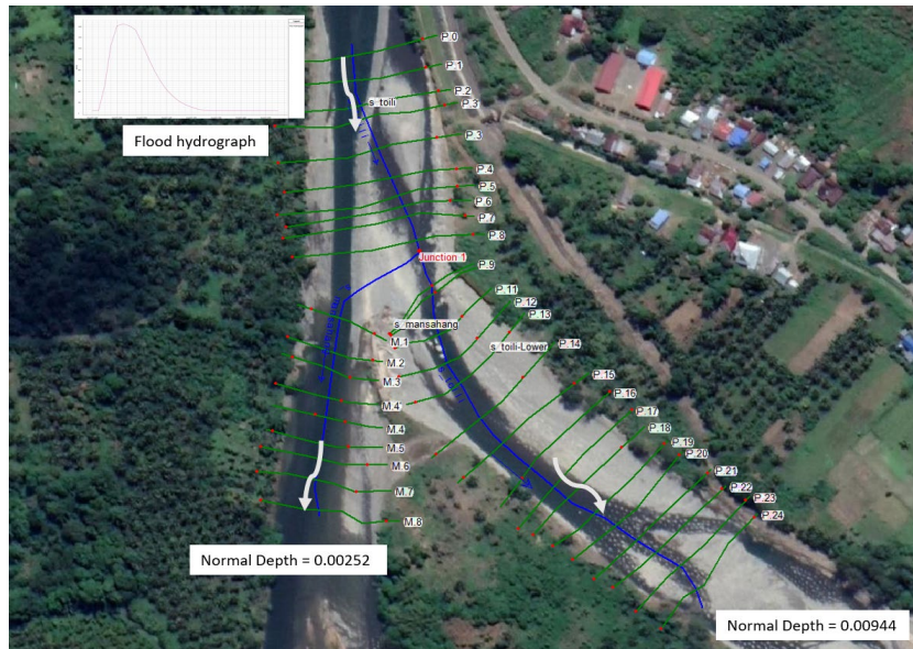
Figure 10. Simulation boundary conditions
